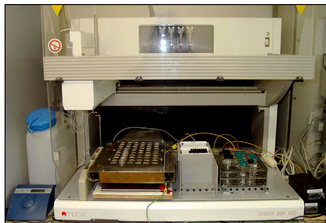
Fig. 1. The HTE workstation equipped with a 60-wells reaction block.
